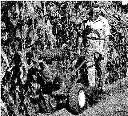
(1) Make first pass alongside first row with RIGHT wheel up close to, but not touching any cornstalk. The purpose of this pass is to loosen up soil in preparation for next pass.
